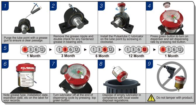
Note • The periodic checkup is necessary when lubrication points are located outside or expected to be infiltrated by water, moisture & humidity. • Dispensing rate may vary according to the grease types, the ambient temperature & conditions of lubrication points.
