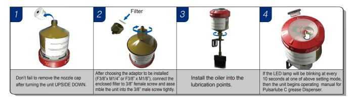
Note · When re-installment is required, Make sure that the filter as well as oiler should be replaced.
